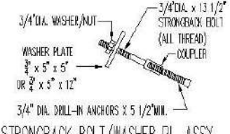
STRONGBACK BOLT/WASHER PL. ASSY.
